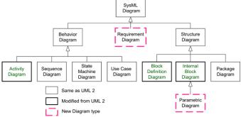
Figure 2 - Diagram relationships between UML and SysML [1]
