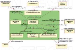
Figure 9 - Detailed Software Design [8]
