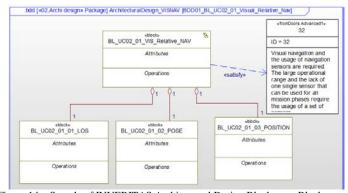
Figure 14 – Sample of INVERITAS Architectural Design Blocks as a Block Definition Diagram (BDD) [10]
